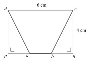
Find the distance of the centre of gravity of the shape *abcd* from |ab|.
